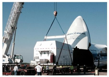
Offloading the SSL-built AsiaSat 6 spacecraft from a transport aircraft at Cape Canaveral
